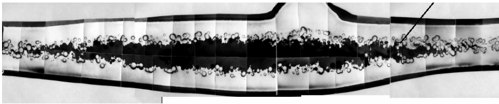
Fig.4: Cross section of failed U-Mo fuel tube from testing in the IVV-2M reactor.
