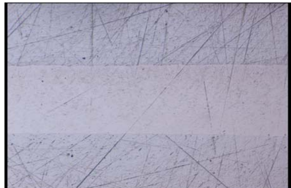
Fig.8a & 8b: Monolithic fuel plates with alternate interface designs after irradiation to ~80% and ~50% LEU equivalent burnup, respectively; (a) shows the fuel/clad interface in a fuel plate fabricated by TLPB with a high silicon interaction layer and (b) a zircaloy clad monolithic fuel plate after irradiation.
